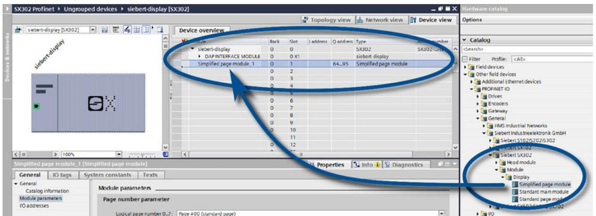
The screenshot shows the 'Hardware catalog' on the right and the 'Device overview' table in the center. A blue circle highlights the 'Simplified page module' in the catalog, and another blue circle highlights the same module in the device overview table. A blue arrow points from the catalog to the table. The device overview table has the following data:
